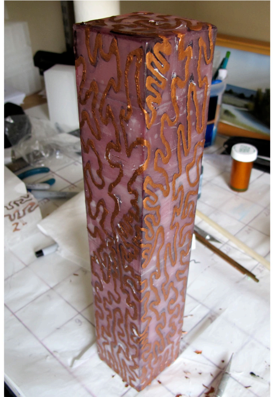
46 Clear red plastic rectangular solid after thin coating of wax then pattern redrawn on surface (left). Labyrinth line painted with conductive paint. Process was unsuccessful – probably due to poor conductivity of the paint.
