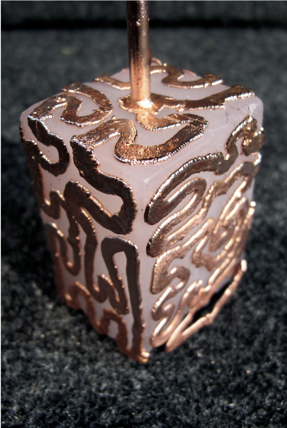
Examples of electroformed mandrels investigating different channel shapes and plating methods. 17
