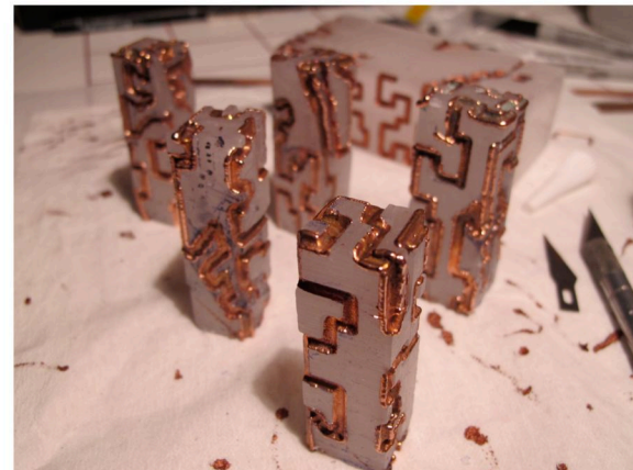
Six individual substructures for sculpture after electroforming prior to wax burnout (left). Finished sculpture titled WRITE Hand (above and detail on facing page).
