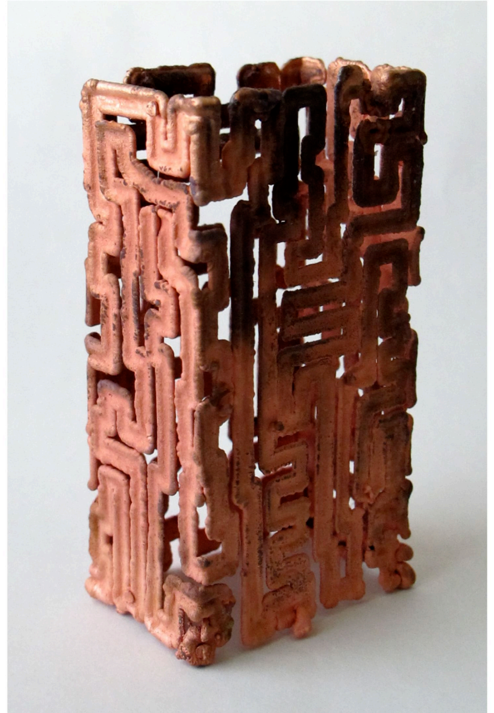
Wax mandrel for Labyrinth 110501 after milled and painted channels. Note multiple electrodes to promote conductivity (left). Same piece after electroforming - wax melted away not burned (right).
