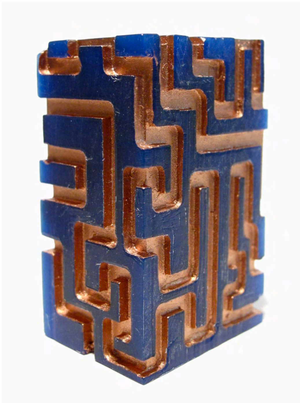
Milled, painted, and cleaned-up wax hull ready for electroforming.
