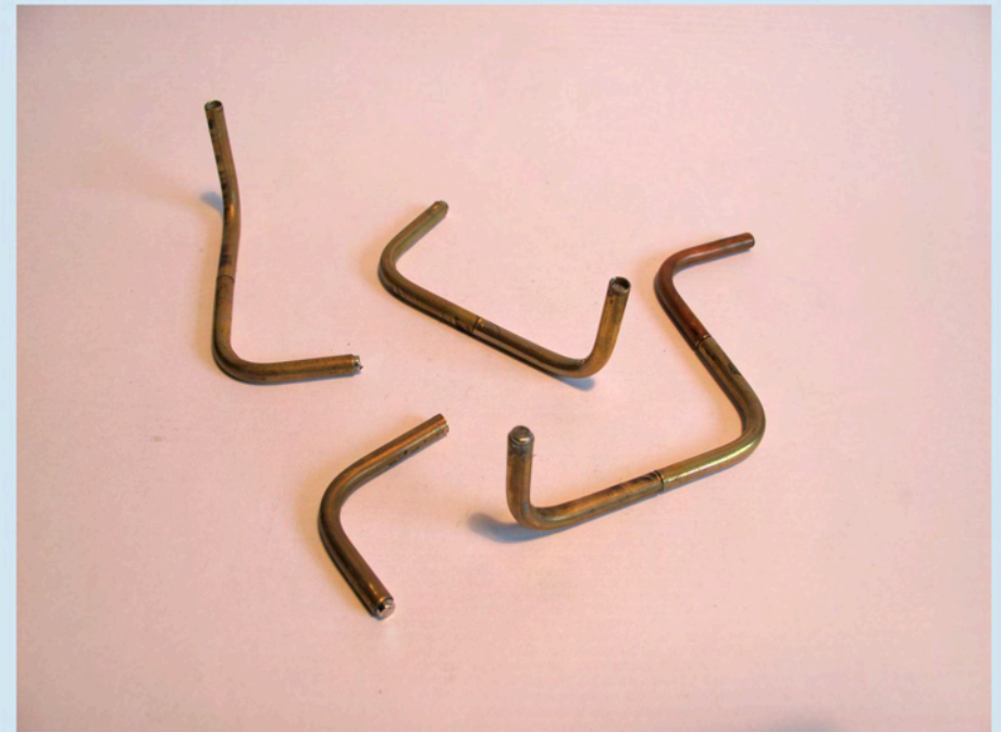
Process explorations led to the design of several tools such as this system of 90° elbows that can be used to construct Hilbert -inspired forms. The elbows have magnets in the ends which keep the pieces firmly, but non-permanently connected.
