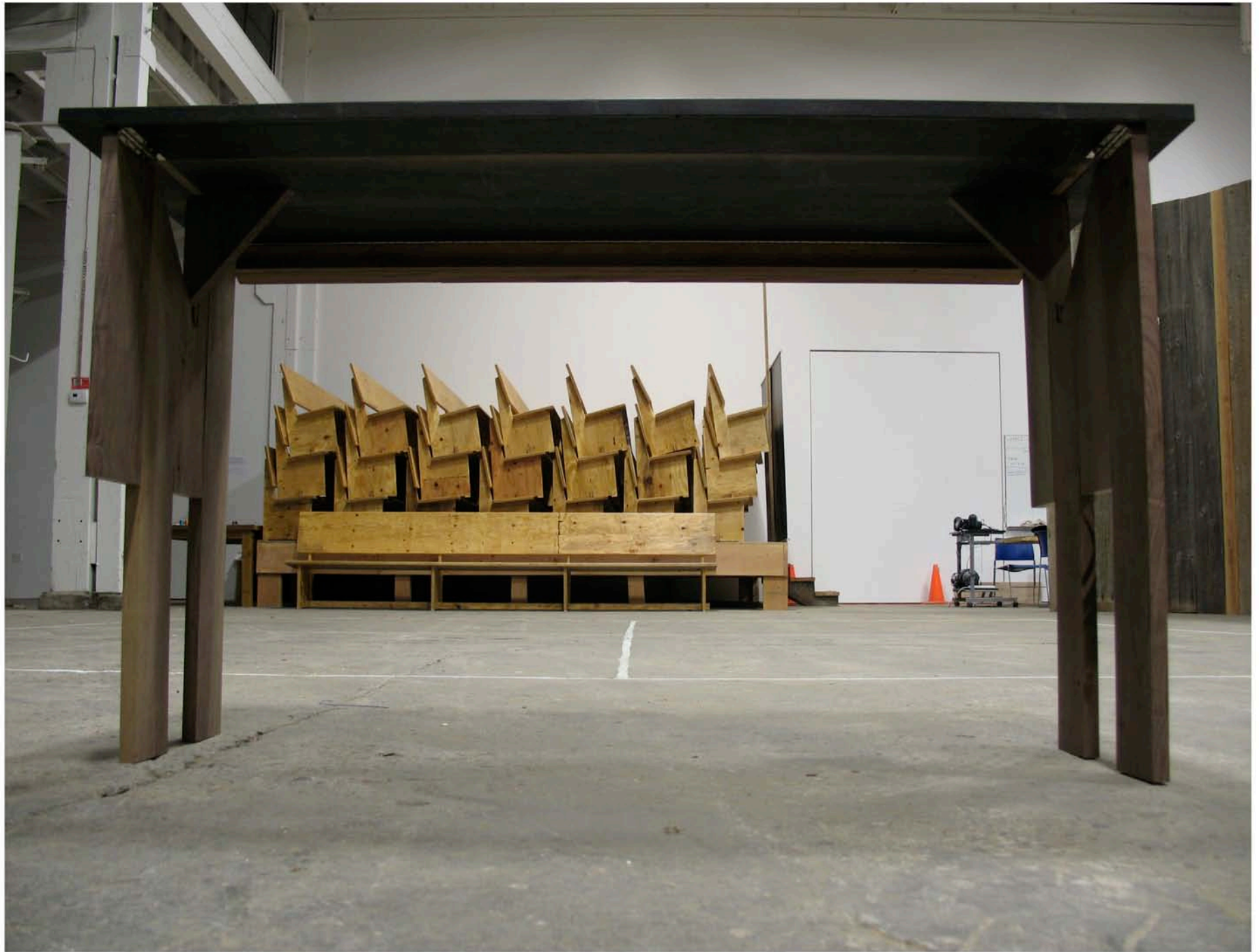
Detail of flip-in lateral stabilizers for legs.
