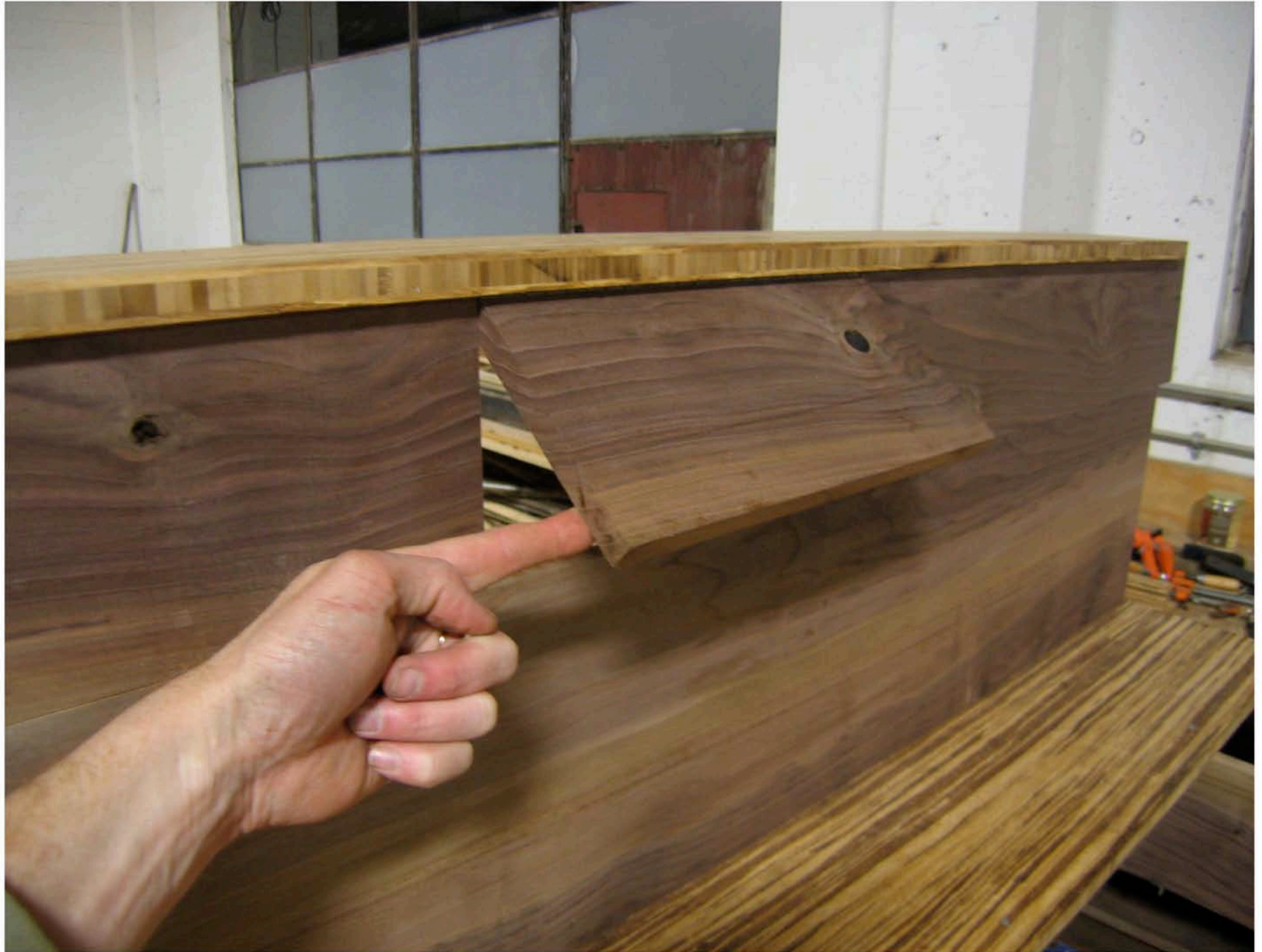
Construction detail: secret stash in headboard.
