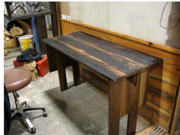
The finishing process: sanding and linseed oil - lots of both.
