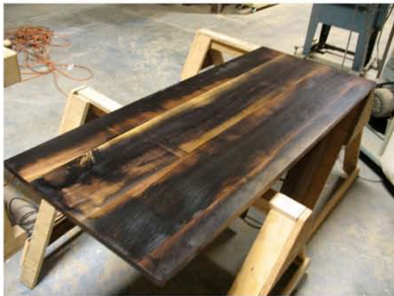
The finishing process: sanding and linseed oil - lots of both.
